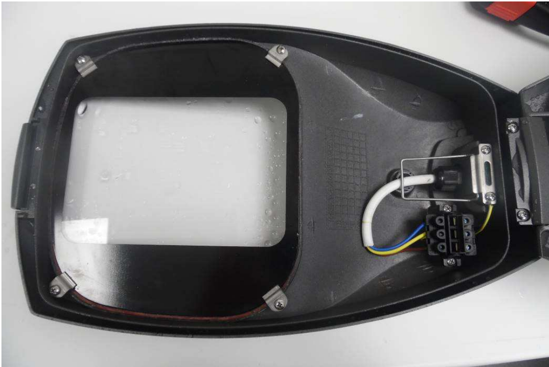
Inside the EUT (post IPX6 test)
