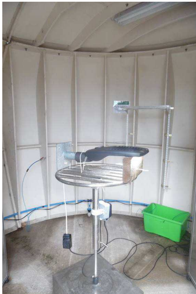
IPX6 test setup
