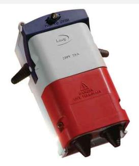
Double pole, single fuse, street lighting cut out for looping up to 6mm <sup>2</sup> 3 core swa cables (when used with a BW gland). Complete with brass cable entry plate with 2 x 20mm holes. Length 150mm, width 81mm, depth 65mm. Rated at 25A maximum. Manufactured & tested to BS7654.
