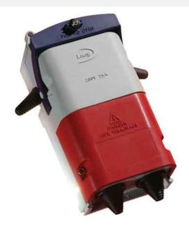
Double pole, single fuse, street lighting cut out for looping up 2 to 6mm 3 core swa cables (when used with a BW gland). Complete with brass cable entry plate with 2 x 20mm holes. Length 150mm, width 81mm, depth 65mm. Rated at 25A maximum. Manufactured & tested to BS7654.
