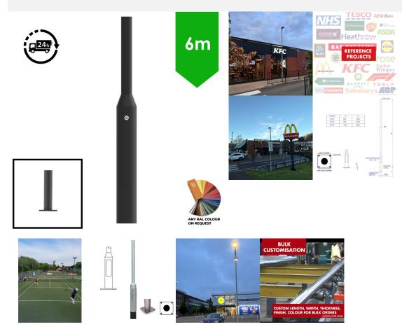
Flange Plated Lighting Column 6m (Bolt Down) - Steel Galvanised Tubular Street Lamp Post (76mm Shaft / 140mm Base) c/w with door (500mm x 100mm) and wooden backboard/ Column Weight 47kg. Maximum head load (kg/m2) = 20 / 0.40. Hot dipped galvanised. Light duty lighting column suitable for road, residential, CCTV/security features and general amenity areas, with street lanterns, floodlights & post top amenity luminaires (please see related accessories).
