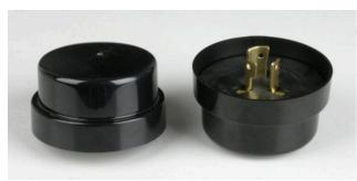
The shorting cap used to replace a NEMA socket photocells when continuity between Li and Lo is required (eg for testing or to make a lantern operate 24/7)
