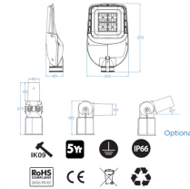
LED Eco Street Lantern Light DIMENSIONS
