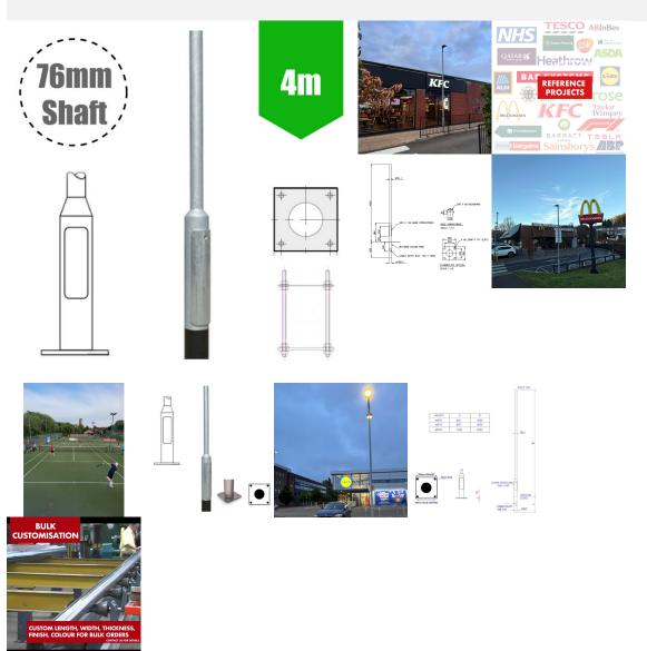
Flange Plated Lighting Column 4m (Bolt Down) - Steel Galvanised Tubular Street Lamp Post (76mm Shaft / 140mm Base) c/w with door (500mm x 100mm) and wooden backboard/ Column Weight 32kg. Maximum head load ( Kg/m2) = 25 /0.5 for terrain category 3. Hot dipped galvanised. Light duty lighting column suitable for road, residential, CCTV/security features and general amenity areas, with street lanterns, floodlights & post top amenity luminaires (please see related accessories)
