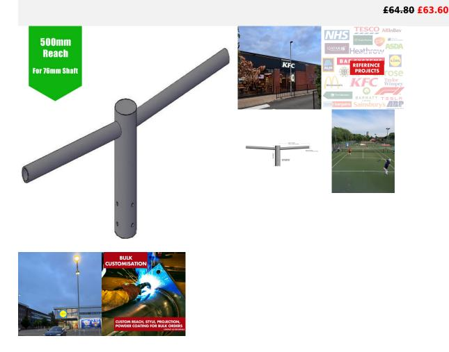
Lighting Column Arm -Twin / Double Projection Bracket 500mm Bracket 60mm Arm Diameter - Steel Galvanised Post-Top for 76mm Shaft column entry. Supplied complete with 4 x M10 Grub screws for securing to the column shaft. **PLEASE NOTE -Weight & Windage must be checked for suitability of the bracket against the installation postcode. Please email us for more information prior to purchase.**
