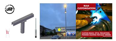
Lighting Column Bracket - Twin / Double Floodlight Bracket - Steel Galvanised Post-Top for 76mm Shaft column entry. Supplied complete with M16 Bolt/Tapped hole for fixing the the flood light & 4 x M10 Grub screws for securing to the column shaft. PLEASE NOTE - Weight & Windage must be checked for suitability of the bracket against the installation postcode. Please email us for more information prior to purchase.
