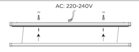
Install plastic plugs into the drilled holes. Feed the cable from the backside of the fitting. Using the screws install the backside of the fitting on the wall/surface.
