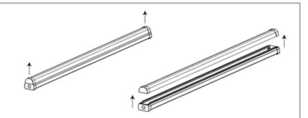
2. Press the sides of the base and gently remove the front cover/diffuser. LED Batten Fiiting has safety straps inside for hads free maintenance.
